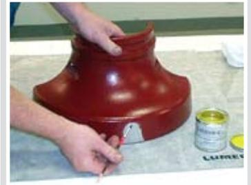
The primer is applied on the cleaned surface
